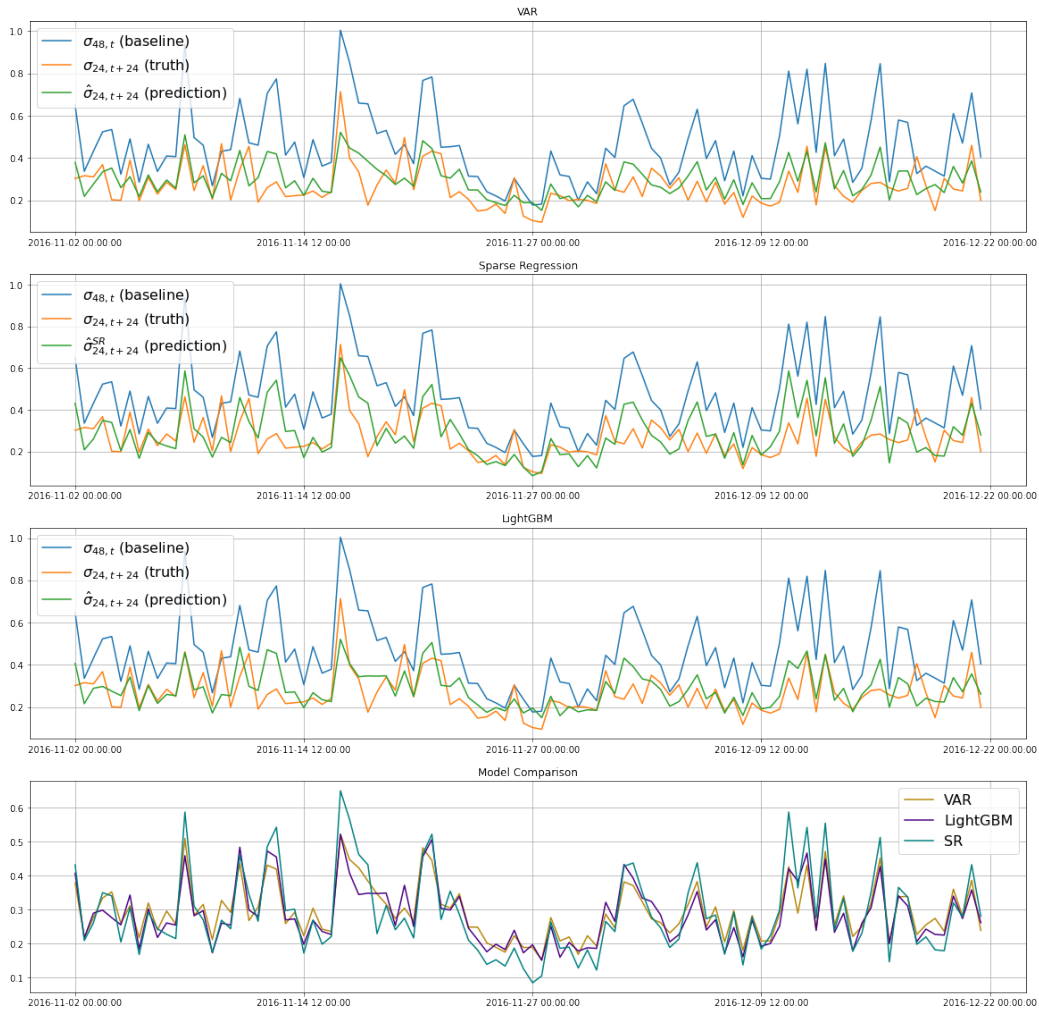
Figure 4: Ahead of predictive modelling, our knowledge of physical model uncertainty, and therefore weather uncertainty was limited to forecasts at time t : \sigma_{48,t} , our uncertainty from 48 hours out. Our prediction \hat{\sigma}_{24,t+24} uses only knowledge available at time t and represents an understanding of the uncertainty from t+24 , narrowing the uncertainty by over 30 %.
